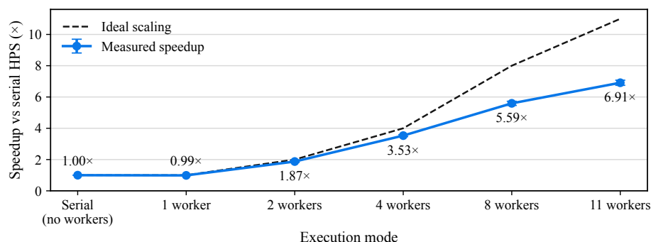
FIGURE 14. Thread scaling of cost-aware HPS on 10,000 puzzles, relative to serial HPS without workers. Points show mean paired per-round speedups over five rounds; error bars show one sample standard deviation. The dashed line shows ideal linear scaling.
